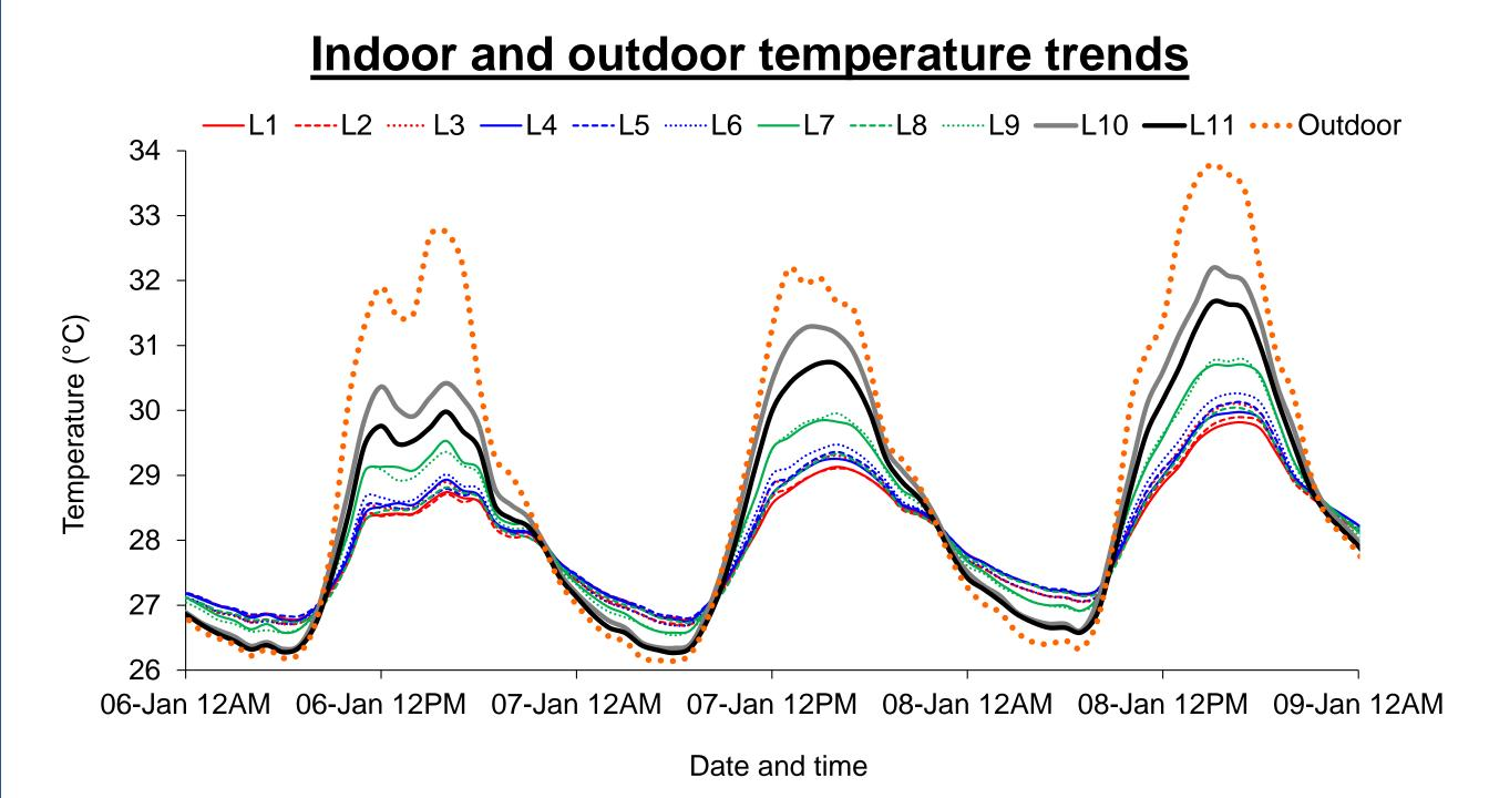
The indoor temperature trend follows that of the outdoor temperature, with peak temperatures in the afternoon and lowest temperatures in early mornings
