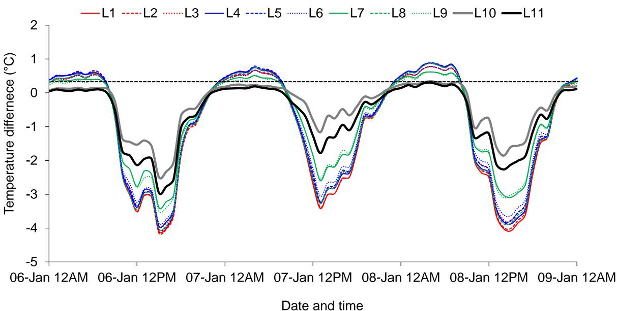
During daytime, the indoor temperature can be up to 4 °C lower than the outdoor temperature, while nighttime indoor temperatures align closely with outdoor.
